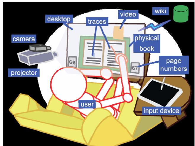
**Figure 1.** A camera captures the user's finger gestures on the desktop and book. These finger movements are used to access digital media. An input device is used to enter new annotations, which results in new traces being displayed.
